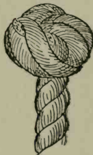
FIG. 123.—Double wall (complete).
